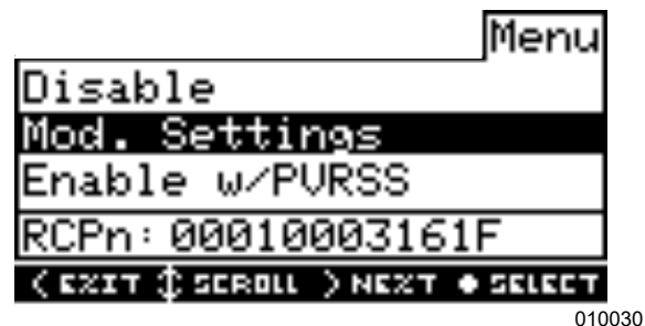
Figure 6-2. PVRSS Commissioning (1 of 4)
