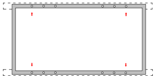
Outer four holes installation method (L-O)
