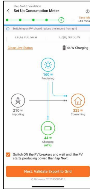
Switch ON the PV breaker to verify if the consumption reading is decreasing
