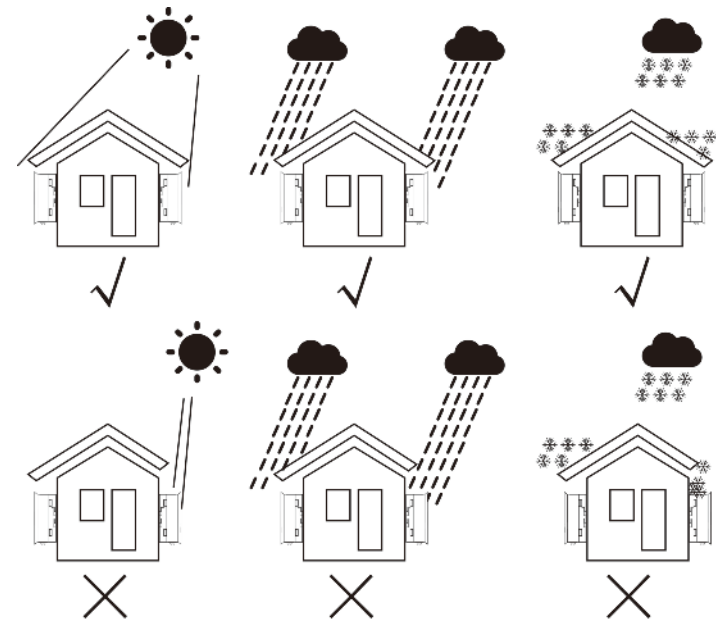
▲ Figure 4.1 Recommended installation position
