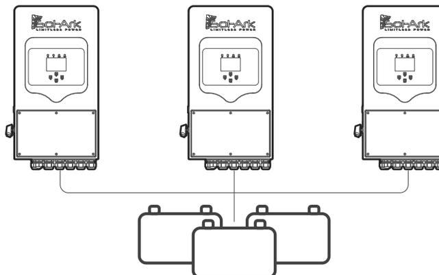
Figure 6: Single battery bank for parallel inverters
