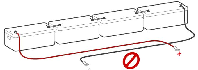
⚠ **DO NOT** reverse polarity. The system will be damaged, and warranty will be voided!
