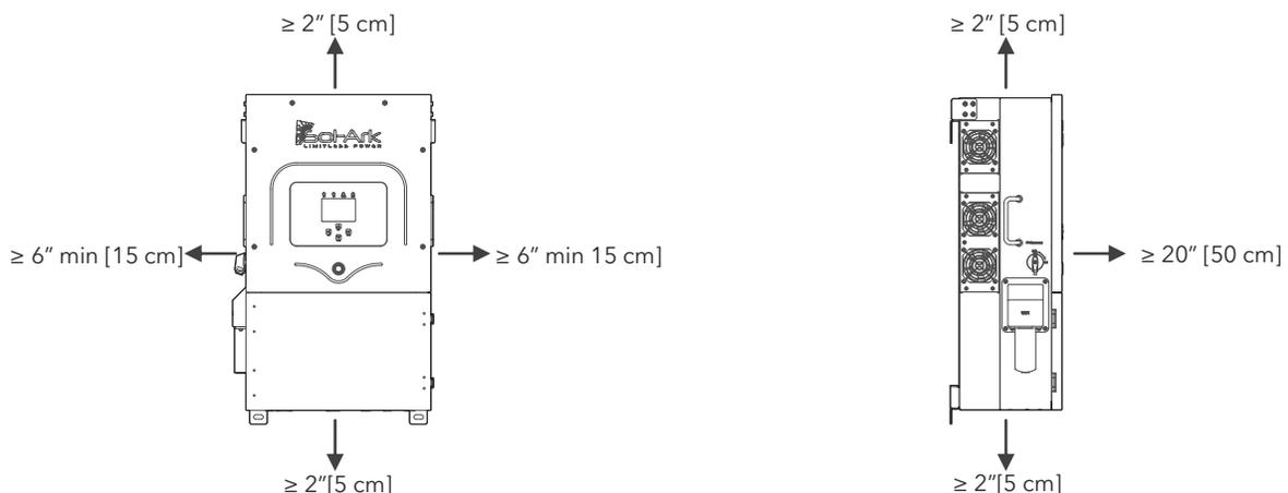
! Max heat dissipation of 175W
