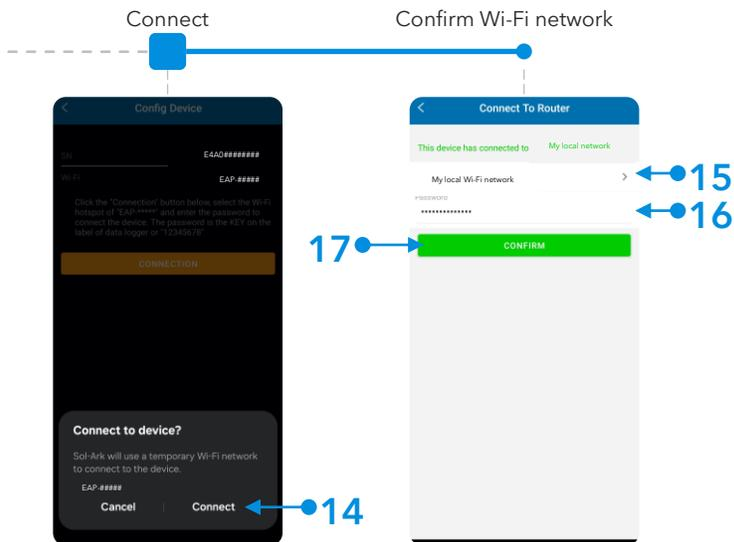
**NOTE:** The Wi-Fi configuration tool can be accessed at any other time by tapping “Me” at the bottom right corner, then “Tools” and finally “Wi-Fi configuration”. STEP 3 shows an alternative method of connecting the Wi-Fi dongle to a local network through an IP address.
