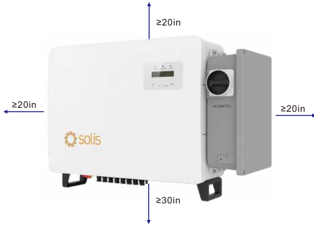
Figure 3.2 Clearance distances requirement for the inverter
