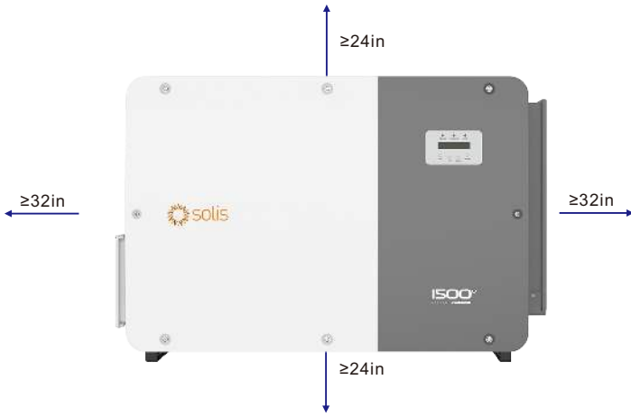
Figure 3.2 Clearance distances requirement for the inverter
