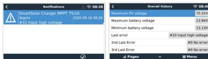
GX device showing alarm notification and historic errors.
