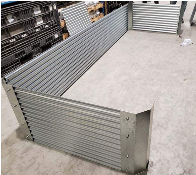
Fig. 1 –Tub Assembly with one Long Side Panel Installed
