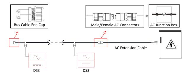
When AC extension cable is needed, users could connect the AC bus cable and AC extension cable in a junction box or use a pair of male/female AC connectors that APsystems provides as optional accessory.
