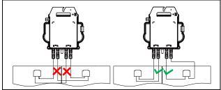
NOTE: When plugging in the DC cables, the microinverter should immediately blink red one time and green ten times. This will happen as soon as the DC cables are plugged in and will show that the microinverter is functioning correctly. This entire check function will start and end within 10 seconds of plugging in the unit, so pay careful attention to these lights when connecting the DC cables.
