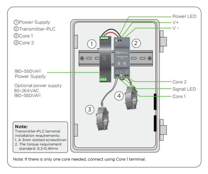
The power supply of the Transmitter-PLC and the inverter must be on same AC branch circuit as inverter to meet rapid shutdown requirements.
