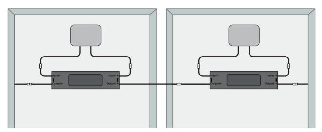
Step 3: Connect the output ports of two adjacent RSD-S-PLCs in series and then connect to the inverter with a self-made DC extension cable.
