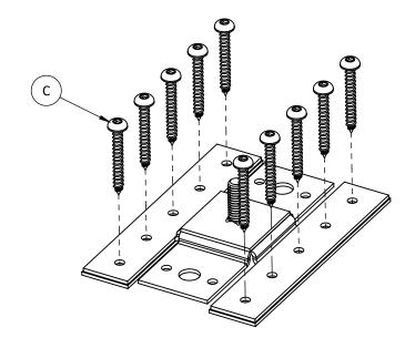
The Talon may also be installed directly to the roof truss using structural lag screws. Two screws are installed using the larges center holes on the Talon Base.
