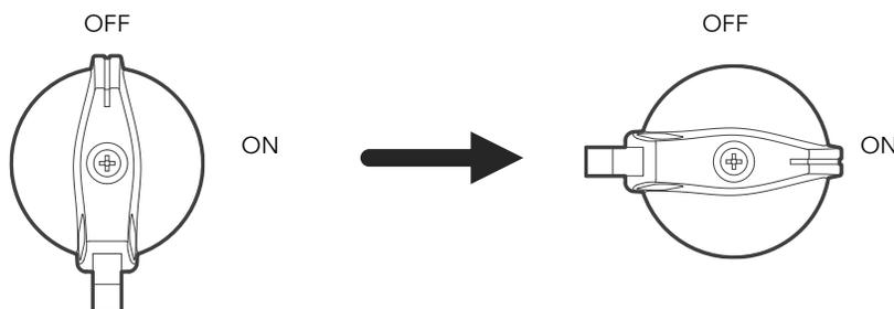
Figure 20: Built-in PV DC disconnect
