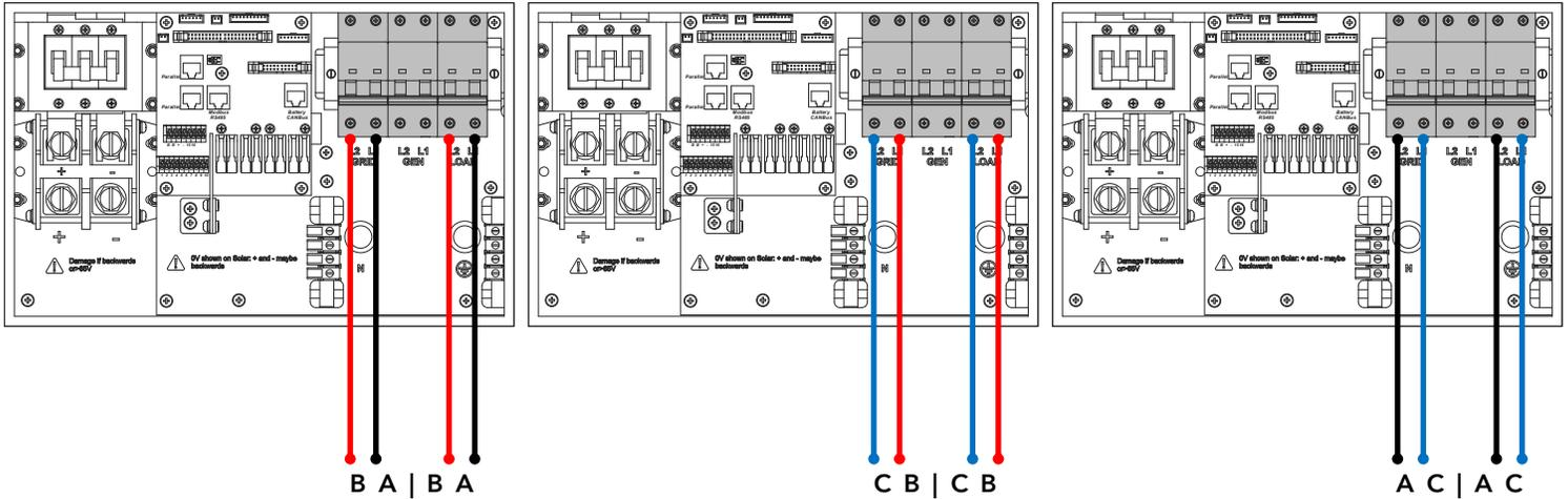
Figure 38: Example of correct phase sequence
