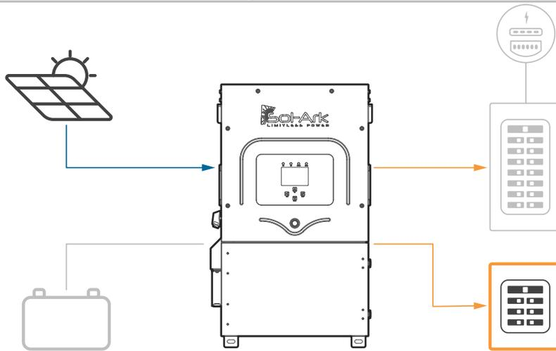
Figure 30: Limited Power to Load + Grid Sell
