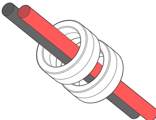
Figure 6: Battery toroid installation
