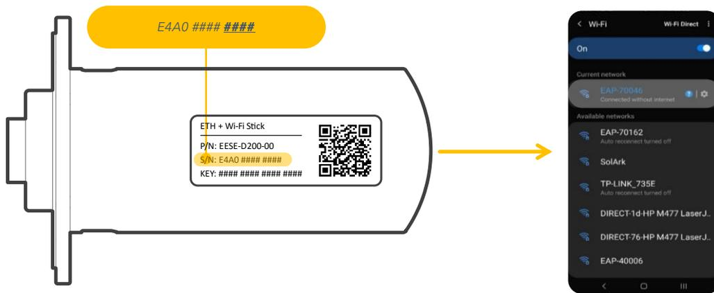
Figure 41: E4A0-##### serial number and EAP network
