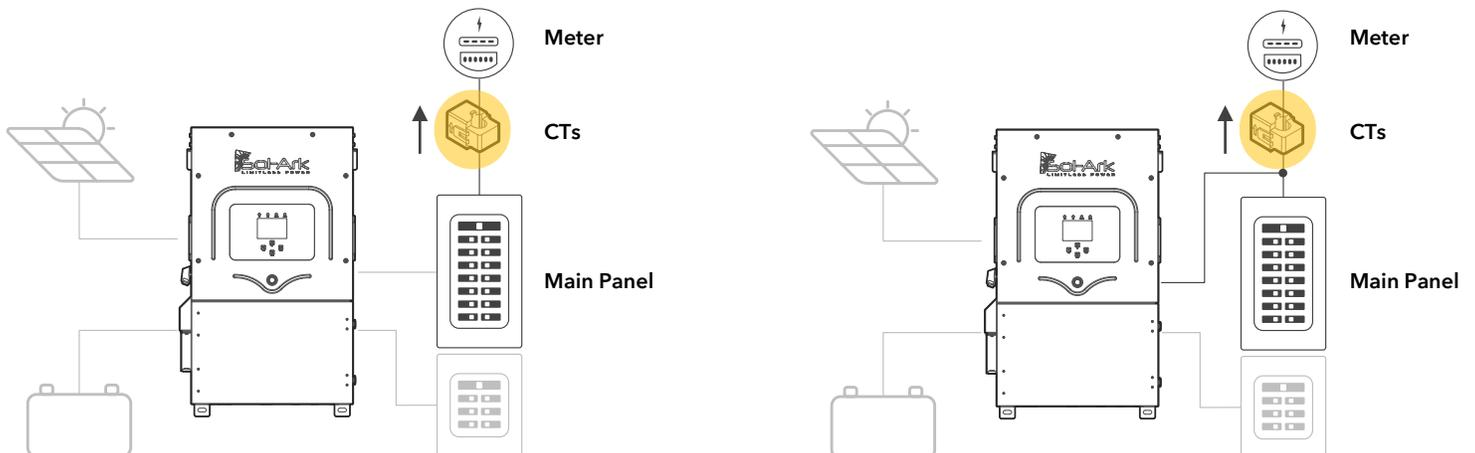
Figure 16: Installation of CTs for a) back-feed breaker and b) line side tap
