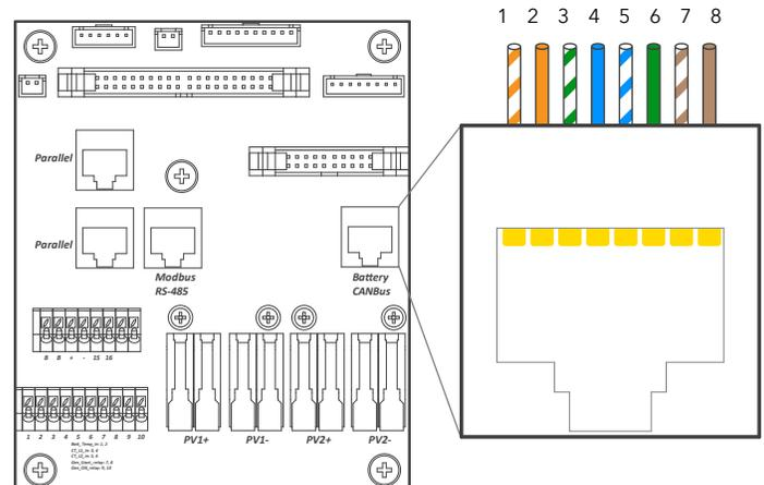
Figure 33: RJ-45 port configuration
